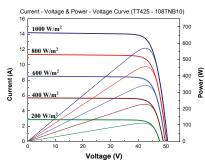
\*Note 1: The specifications are obtained under the standard test conditions: 1000W/m2 solar irradiance, 1.5 Air Mass and cell temperature of 25°C. Measurement uncertainty for all panels is 6%. The actual transactions will be subject to the contracts. These parameters are for reference only and it is not a part of the contracts. The specifications are subject to change without prior notice.
