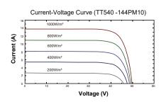
\*The specifications are obtained under the standard test conditions: 1000W/m2 solar irradiance, 1.5 Air Mass and cell temperature of 25°C. Measurement uncertainty for all panels is 6%. The actual transactions will be subject to the contracts. These parameters are for reference only and it is not a part of the contracts. The technical specifications in this document may vary. For more information, refer to the "Installation Manual".
